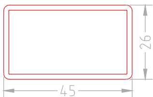
BF 426-12 (Thickness 1.2mm) BF 426-15 (Thickness 1.5mm) BF 426-20 (Thickness 2.0mm)
