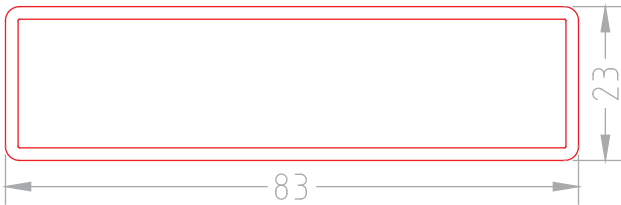
BF 425-12 (Thickness 1.2mm) BF 425-15 (Thickness 1.5mm) BF 425-20 (Thickness 2.0mm)
